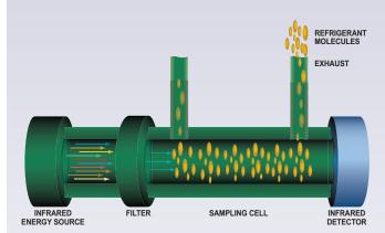
Filtered infrared energy is absorbed by the refrigerant present in the sampling cell, causing D-TEK Select to alarm.
